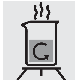
Evaporate 200 ml of sample solution in a glass beaker almost to dryness on the hob.
