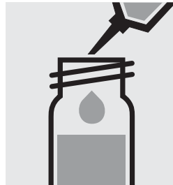
Add 5.0 ml of distilled water with pipette, close with the screw cap, and mix.
