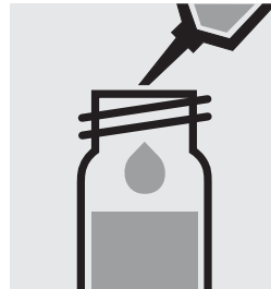
Pipette 0.50 ml of the sample into a reaction cell, close with the screw cap, and mix.
