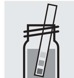
Check the pH, specified range: pH 10.0–11.5.
